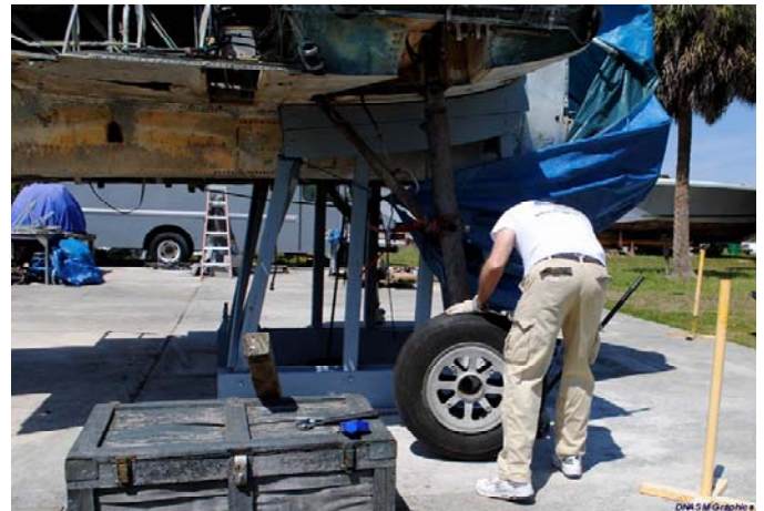
With Oleo Strut partially collapsed Wheel is then trial fitted.
