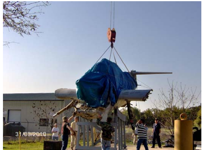
TBF off slab, cradle is put in position, TBF is lowered down
