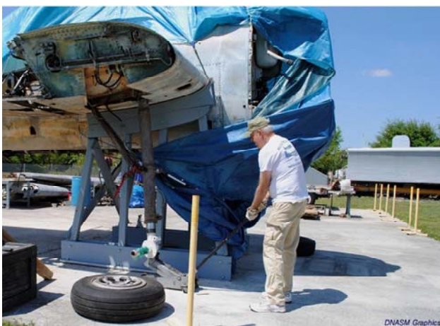
Cal collapses Oleo Strut to Raise spindle for wheel
